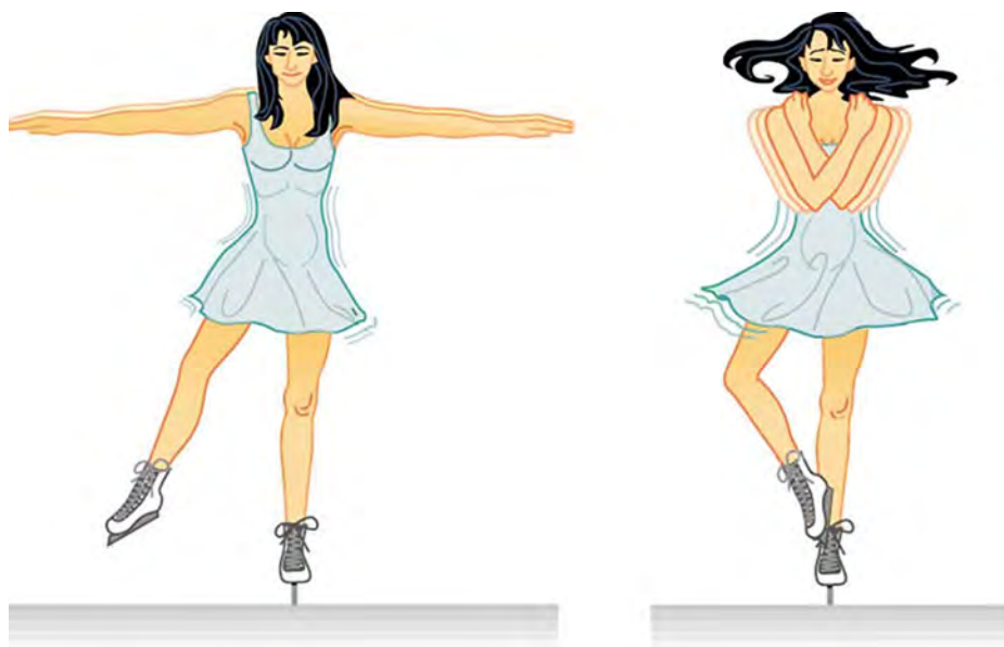
Figure 3.8. Conservation of Angular Momentum. When a spinning figure skater brings in her arms, their distance from her spin center is smaller, so her speed increases. When her arms are out, their distance from the spin center is greater, so she slows down.
