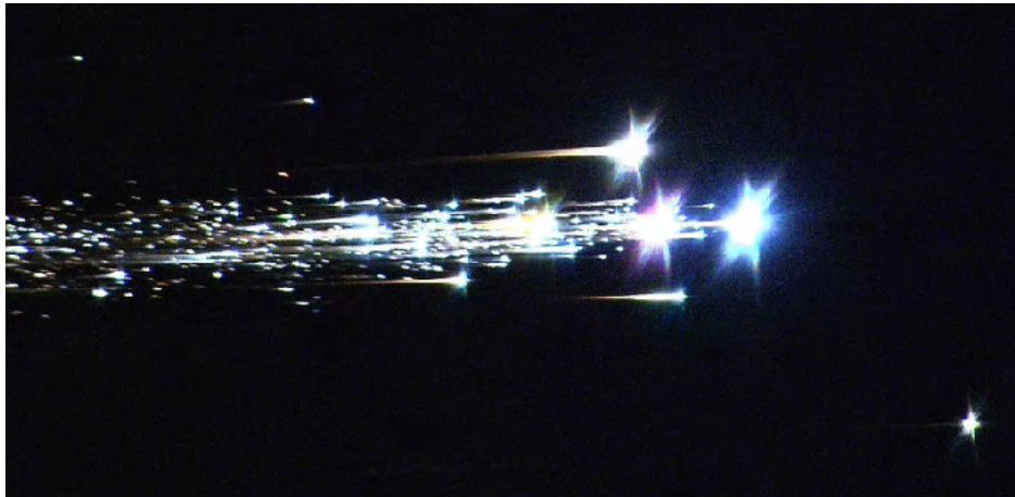
Figure 13.10. Hayabusa Return. This dramatic image shows the Hayabusa probe breaking up upon reentry. The return capsule, which separated from the main spacecraft and parachuted to the surface, glows at the bottom right. (credit: modification of work by NASA Ames/Jesse Carpenter/Greg Merkes)
