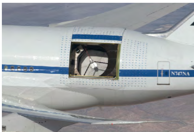
Figure 6.23. Stratospheric Observatory for Infrared Astronomy (SOFIA). SOFIA allows observations to be made above most of Earth's atmospheric water vapor. (credit: NASA)
