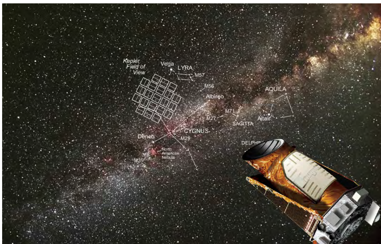
Figure 21.20. Kepler's Field of View. The boxes show the region where the Kepler spacecraft cameras took images of over 150,000 stars regularly, to find transiting planets. (credit "field of view": modification of work by NASA/Kepler mission; credit "spacecraft": modification of work by NASA/Kepler mission/Wendy Stenzel)
