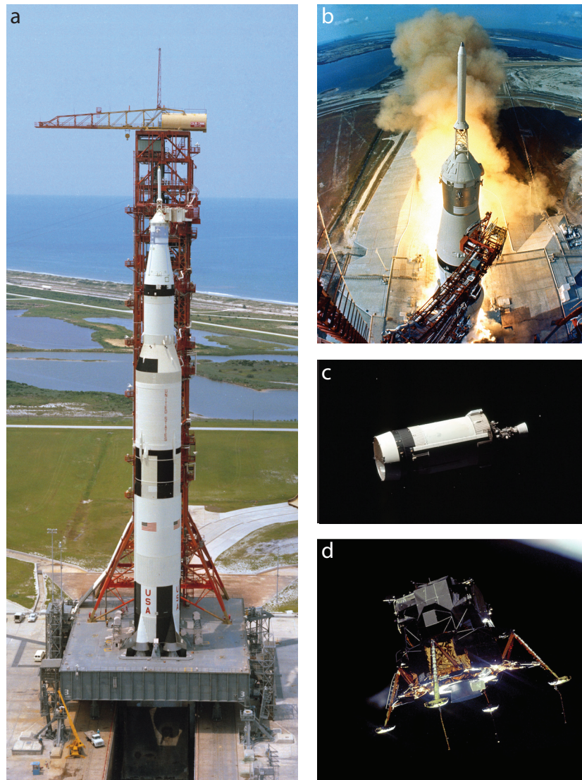
Figure 4.3: Rockets and related spacecraft that took people to the moon in the late 1960's and early 1970's [15]. (a) Aerial view of a Saturn V rocket on its launchpad. This rocket carries the Apollo 15, the fourth mission to make it to the moon. The three rocket stages are separated by rings around the engine of the next stage. The total height of the rocket at launch was 110.6 m; it had a total mass of 2.97 million kg, and could take a payload of 140000 kg to low-Earth orbit or a payload of 48600 kg to the moon. (b) View from the launch tower of the Saturn V carrying Apollo 11 (the famous first mission to the moon in 1969) at ignition. The little rocket on top was to be used for an emergency escape of the manned module immediately below if anything went wrong at launch. The manned 'command module' is the little conical structure; the cylindrical structure directly below it contained its engine, and the conical part below that contained the lunar lander (figure d). (c) Jettisoned third stage of the Saturn V rocket that carried the Apollo 17 mission (the sixth and last(!) to make it to the moon in 1972). The empty space at the front contained the lunar lander module at launch. (d) Lunar lander of the 1969 Apollo 11 mission, photographed from the command module after separation. This module contained two rockets: one to slow the descent to the moon on the lower part, and one to return to moon orbit with just the upper part. The lower part of the lander remains on the moon and was photographed there in 2012 by the Lunar Reconnaissance Orbiter, an unmanned spacecraft in Moon orbit.
